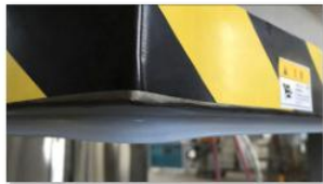
4 VACUUM CHAMBER SEAL STRIP
