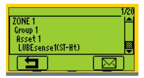
At this point, a message icon is offered in the lower right corner of the display. If the asset is not in operation, or safety is compromised, you have an option to assign a message that explains these conditions and your decision to abort the planned work.
