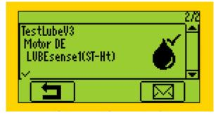
Next position in your work order/survey is Static data measurement of the same asset. Since data has been collected and lubrication task performed, this position is clearly marked as "Done" and you can proceed to your next asset.
