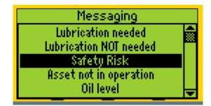
By pressing ENTER, you acknowledge that you are at the RIGHT POSITION at the RIGHT INTERVAL, using the RIGHT LUBRICANT and the RIGHT GREASE GUN. You are also informed if there is an alarm assigned to this position (or not) and if yes, what is the threshold. In case you have multiple alarms, LUBExpert will display lowest (tightest) one that will trigger your decision to apply grease.
