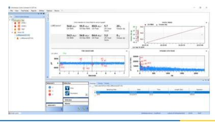
Two Dynamic measurements are collected during initial and final reading of your lubrication process, thus describing condition of your bearing before and after the grease replenishment process. This is great data the lubrication technician provides directly to the condition monitoring team.
