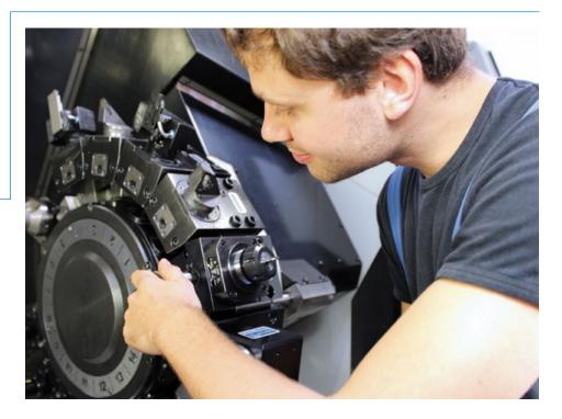
Tool Change for a driven tool with Modular Quick Change System BENZ CAPTO™.
