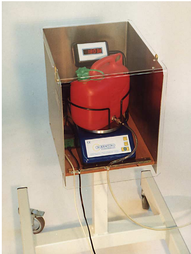
Precision balance with holder securing the tank and with data cable to the MP Computer on a mobile support with wind-break.
