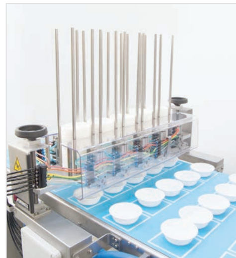
Cup dispenser machine adapted to work in a custard production line
