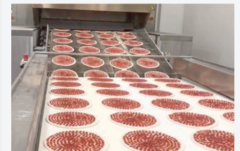
DA filling machine for tomato sauce prepared to be assembled to a continuous pizza working line
