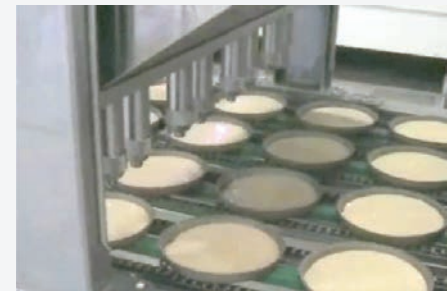
Cup dispenser machine adapted to work in a custard production line
