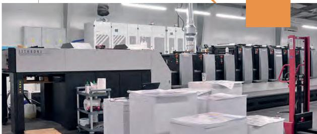
We offer high quality offset and UV offset printing on 6 and 5-colour machines with a coater press. Komori Lithrone GL-629: 6-colour printing with two UV coater presses or dispersion and a drying unit, a machine equipped with automatic systems for correcting ink limit and dot gain.
