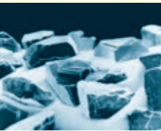
Upon application of an electro-galvanic layer, grit embedding occurs. This provides each piece of grit with the required working space.
