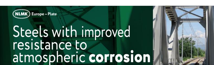
Our weathering steels are produced with a good balanced presence of copper and chromium and can be efficiently integrated in many industrial, architectural or artistic projects. Their structure enables a good regular self regenerating protection layer on the surface. They combine inner high strength with nice natural brown aspect. Their resistance and their aspect make them a cost-effective solution, especially for outdoor use, with or without painting.
