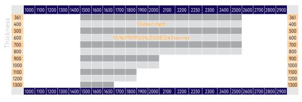
IMPORTANT: the thickness of 1300mm is reached for tool steels and engineering steels. See the specific data sheet for more details
