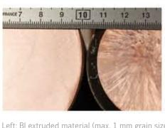
Left: BI extruded material (max. 1 mm grain size) Right: Non extruded - rough continuous casted material (grain size of several cm)
