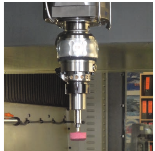
Example: RSC system in a machining centre
