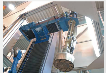
View of Z-Axis with Rasp tool.
