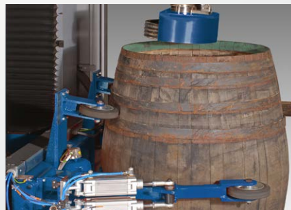
Flexible automatic clamping device for cask.
