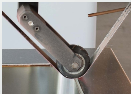
Grinding detail on welded seam with spraying nozzle.
