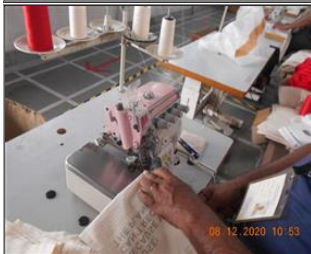
Photo of non-conformity 7.13-Tampered eye guard in sewing machine.jpg
