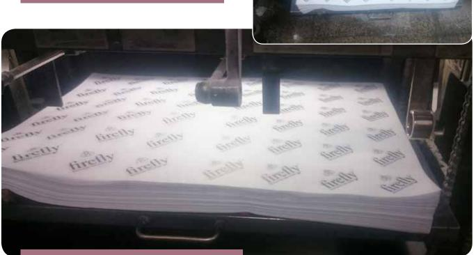
This how the papers look like on the machine after getting printed. Although edges are not bad, they need to be trimmed again for a better quality and easy handling & packaging.
