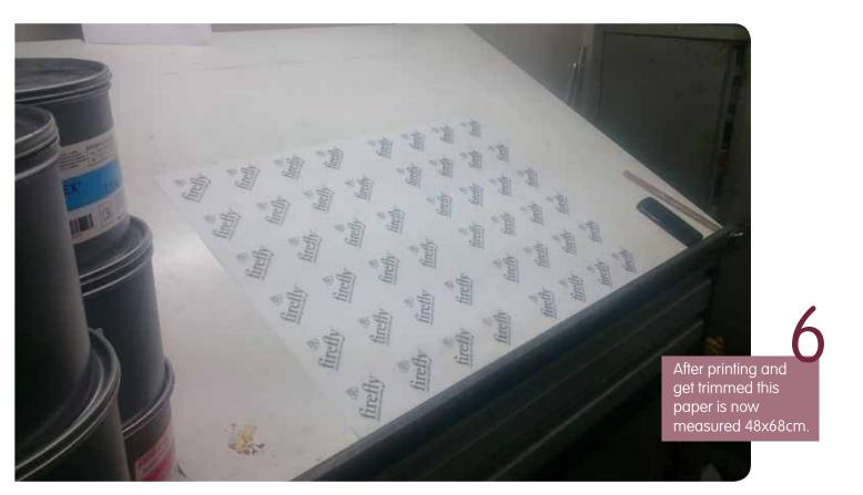
Above you can see the plain area on a printed paper, this area is like about 1cm, needs to be plain, since the machine does not area. For background printed ones or even for the ones with continous design, we need to trim it away. After final trimming the paper is now measured 47x68cm, but to be on the safe side it is better we refer it as 47x67cm.
