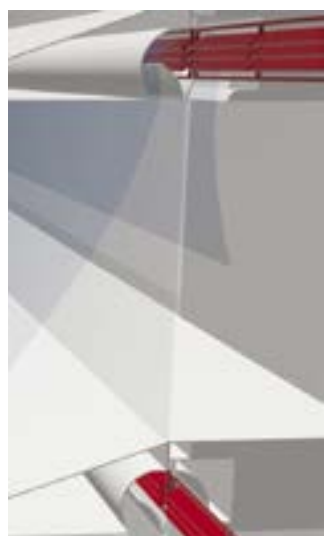
FLW 24 Spiegel Ericusspitze Hamburg: Louvre vents with an insulated panel infill for day-to-day ventilation and heat and smoke exhaust in case of fire, were installed on the roof. Approximately 100 m 2 of vents provides 59 m 2 of aerodynamic ventilation area.
