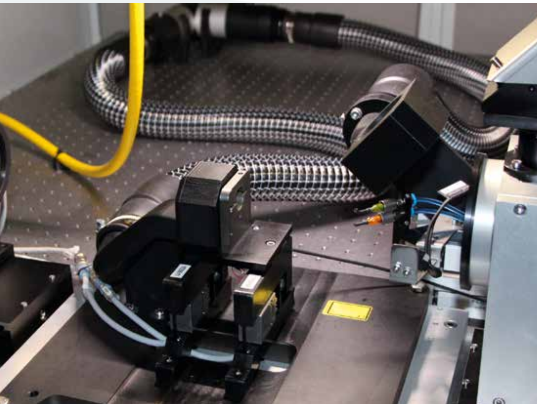
NanoBalancer configuration with two different lasers for two plane balancing. Each laser beam is directed on the respective area of the impeller by a XY scanner with axial orientation of laser beams. The ablation in one plane impacts the imbalance in the other plane so that the amount of the ablated mass needs to be calculated carefully.
