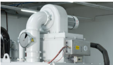
Air heater with blowing nozzles – dries the workpiece
