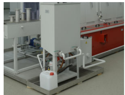
UNI oil separator – separates oils and greases floating up
