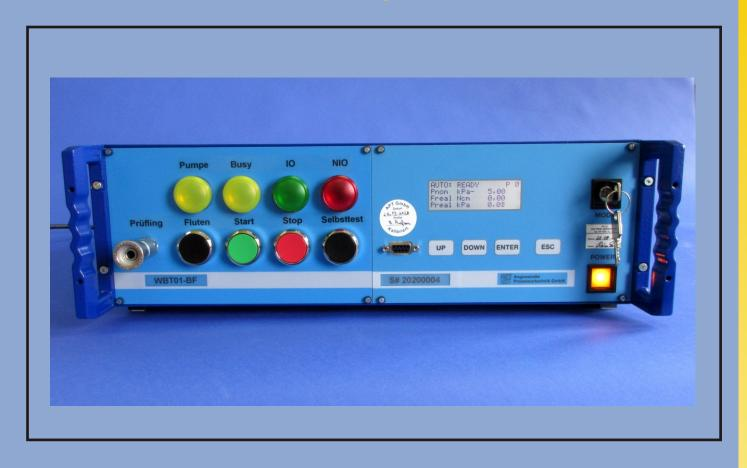
Mass flow leakage test
