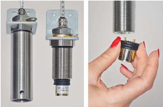
Fig.3. Removing the ISM from the GAOS 5-SD-7031-SM housing
