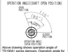
TD100A1 series dampers. Operation angle for TD100B1 series dampers are symmetrical to the
