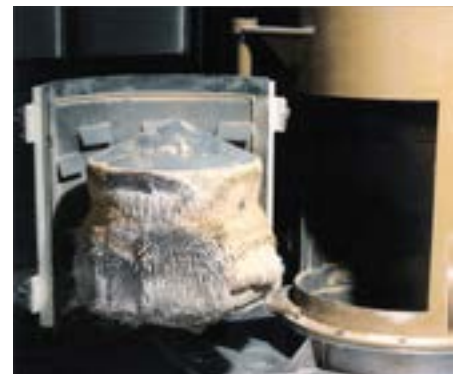
Bullet magnet for ceramic material
