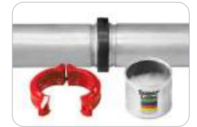
3. Applying lubricant inside of the gasket and the coupling housing
