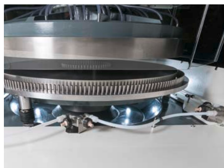
Integrated machine pan rinsing
