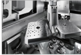
Double gripper for 2 x 150 kg
