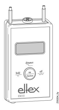
The electric field meter is a parametric amplifier. The charges influenced by the electrical field generate an alternating current proportional to the field strength. This alternating current is measured via a selective amplifier without drawing time-averaged energy from the electrical field. No radioactive substances are used in the instrument.
