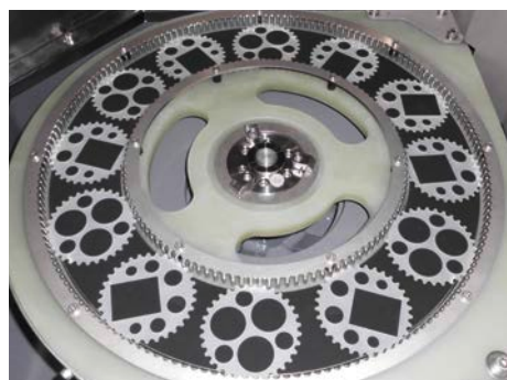
Polishing process with special epicyclic workholder drive for filigree work pieces
