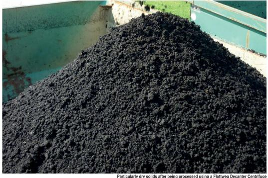
Particularly dry solids after being processed using a Flottweg Decanter Centrifuge
