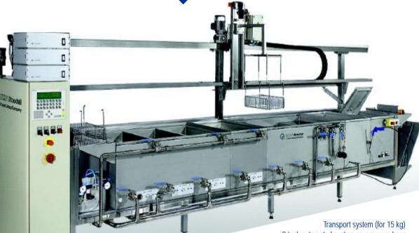
Transport system (for 15 kg) 9 tank automated system on aqueous base type W8-TL1
