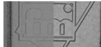
Transparent plastic with embossing - diffuse backlight collimated backlight
