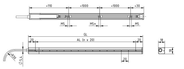
AL = active length 1860 mm max. GL = total length \*M5 depending on length number of sliding nuts M5: AL of 120 - 1000 mm: 2 pieces AL of 1020 - 1860 mm: 3 pieces
