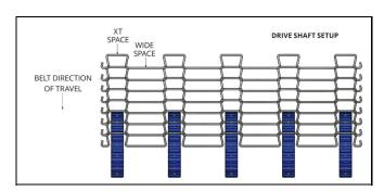
To setup the drive shaft, install one drive sprocket per XT space along the full width of the drive shaft (figure above). Ensure all sprocket teeth are fully aligned.
