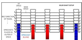
In setting up the idler shaft, install one drive sprocket per outside XT space of your belt (figure above). Then, install one blank on each of the inside XT spaces across the width of the belt. Additional sprockets, interspaced across the width, maybe required for wider belts. Contact Wire Belt Technical Sales for more information.
