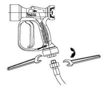
Assemble the inlet tube in the gun, taking care to block with a wrench on hex fitting placed at the base (see image).
