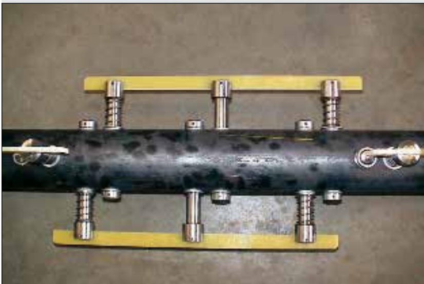
Replacement scraper shaft for paraxylene service
