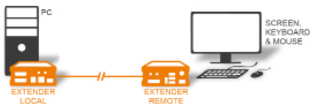
POINT TO POINT CONNECTION
