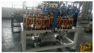
This is 90 series 48 spindle High speed braiding machine mainly used to produce RIC-RAC Lace, Piping Tape, Jacquard Tape, Elastic Band, Fibre Band, Various Rope, Special Band and shoelaces.
