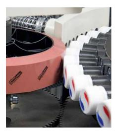
Uneven surfaces do not present a problem, moulding injection points can be overprinted
