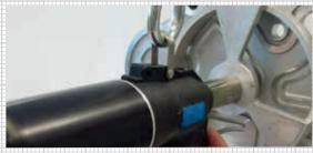
Special accessories: **Angular adapter** to maintain the necessary perpendicularity to the part.
