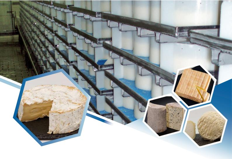
Made of stainless steel or aluminium Materials suitable for heavy products Very high rigidity
