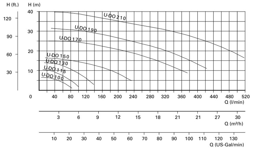
Characteristic lines measured with water, 20° C and 2900 Rpm (50 Hz.)
