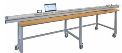
Length measurement on bars
