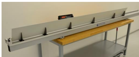
Length measurement on sheet metal strips
