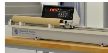
Length measurement on cardboard tubes
