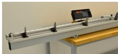
Length measurement on plastic pipes
