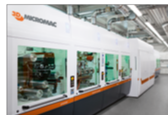
microFLEX™ 300 Laser scribing of organic photovoltaic cells
