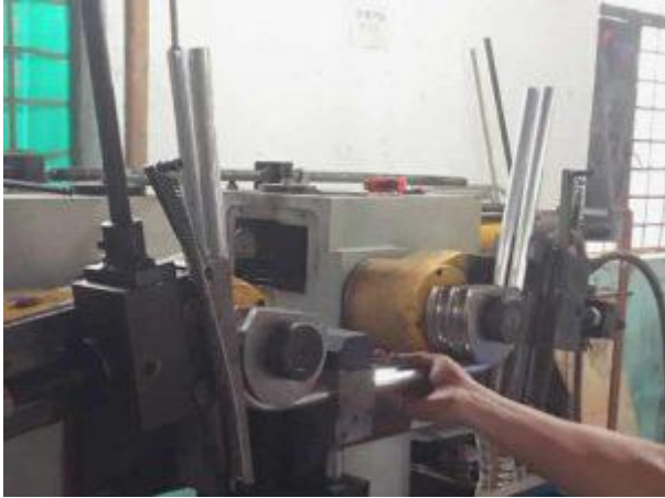
U type Pipe Bending
