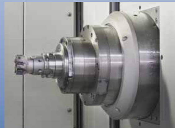
MS 3 integrated in spindle housing
