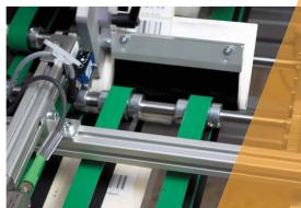
Our HSF-eco model is used for offline labelling of flat products such as empty pharmaceutical boxes, postcards or cardboard blanks. After loading the infeed magazine, the system unstacks the inserted products fully automatically and collects them again after labelling. The system can be refilled during operation and the processed products can be removed. In the basic version, product widths of 350 mm can be easily labelled. Models for processing wider products are optionally available.
