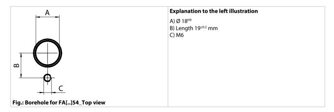
Recommended fixing: Hexagon socket screw DIN912 M6x20 with spring washer.
