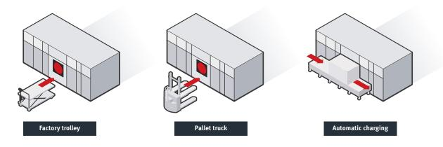
Different types of loading provide flexibility in logistics: factory trolley, fork-lift trucks, automatic loading enable a suitable integration and linking of the plant into the production landscape.
