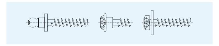
Examples of special parts with REMFORM® F-thread
