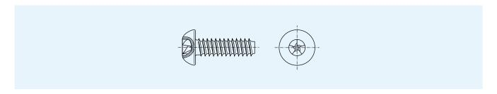
Examples of components with REMFORM® thread
