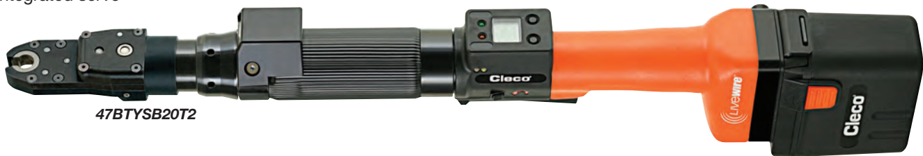
The 47BT tube nut wrench alternates the direction of rotation each time the lever is actuated. When rotating in reverse, the socket will stop at the open position.
