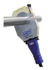
Enclosed weld heads provide complete inert gas protection of the full weld bead circumference (an industry requirement for producing welded joints in electro-polished and hygienic applications).
