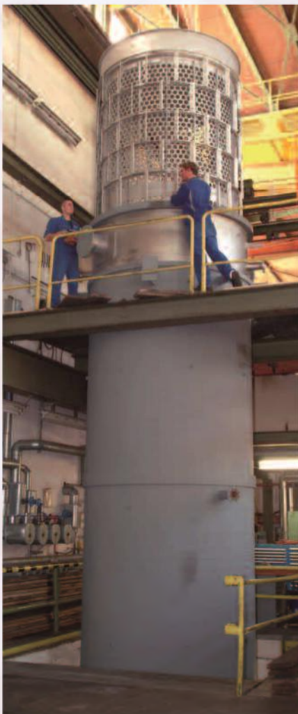
Thin film evaporator in our test facility
